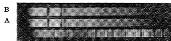
Fig. 6.—The absorption spectra of neodymium chloride (A) and nitrate (B) dissolved in water. (0.476 mol., 1 cm.)
